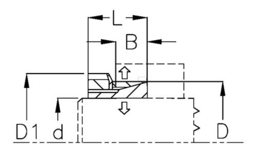
$\begin{array}{lll} \text{B mm} & = 9.0 \\ \text{D1 mm} & = 58 \\ \text{d H8 mm} & = 35 \\ \text{D mm} & = 45 \\ \text{Fit tolerance} & = \text{Aksel h8, Nav H8} \\ \text{F kN torque} & = 15 \\ \text{L mm} & = 22.0 \\ \text{P N/mm2 surface pressure on shaft/hub} = 80 \end{array}$
